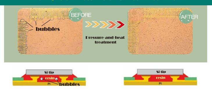
Bubbles disappear after pressure-and-heat treatment
